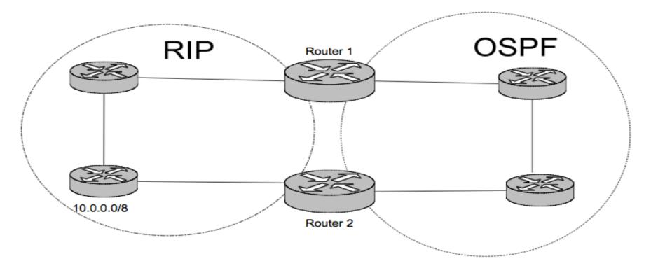
1.Router 1 and 2 are redistributing RIP into OSPF, 10.0.0.0/8 will become OSPF route (E2) 2. Router 2 will use the path through the OSPF network to get to 10.0.0.0/8 because the OSPF route has lower AD. This is not the optimal route
